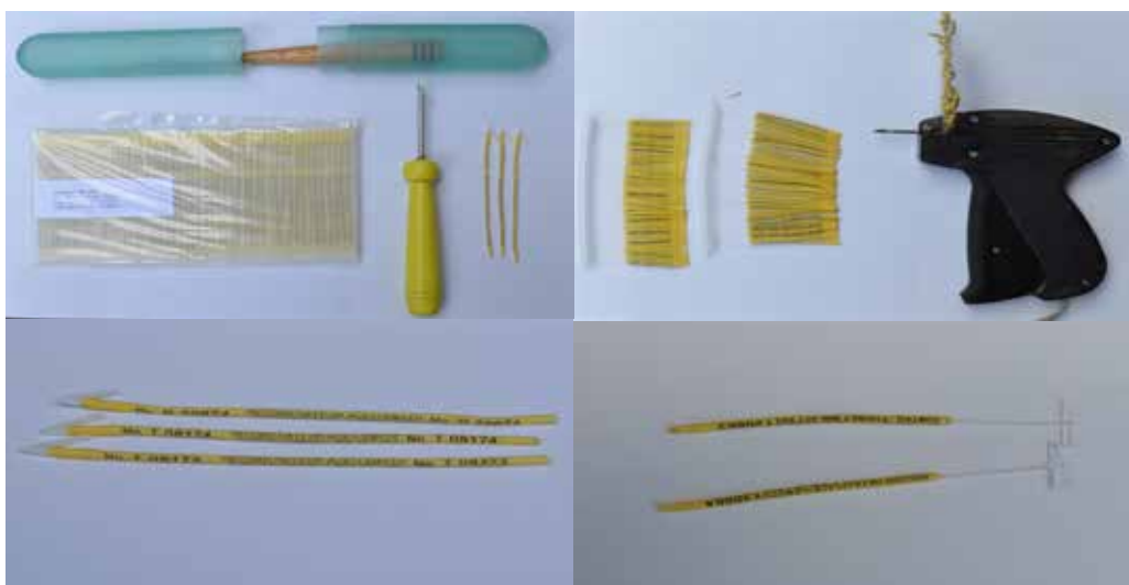
Figure 30: Tags and tagging equipment used in Suntag
